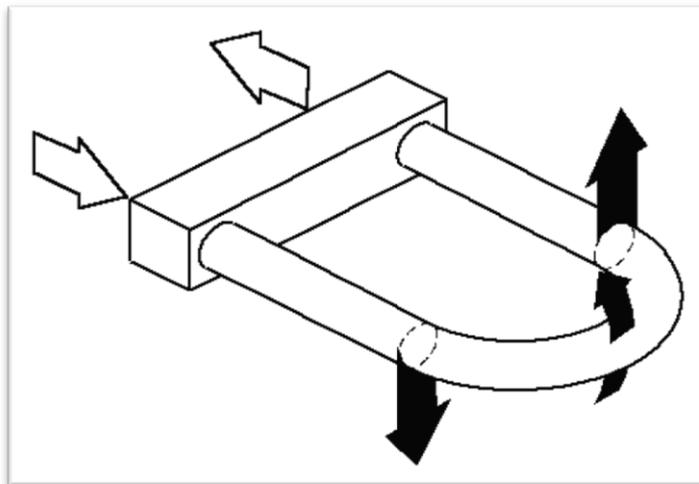
The vibration frequency of measuring tube is determined by the total mass of measuring tube and inner mass flow. The vibration frequency of measuring tube changes over the changes of mass flow density. Thus, the flow density can be calculated.
