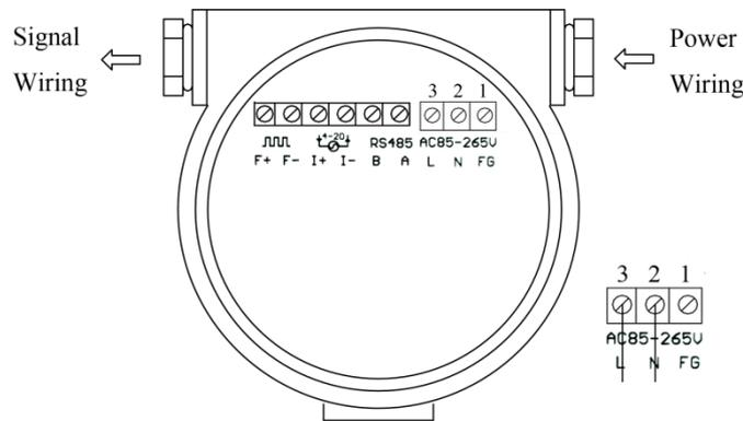
Drawing 13: AC Power Wiring
