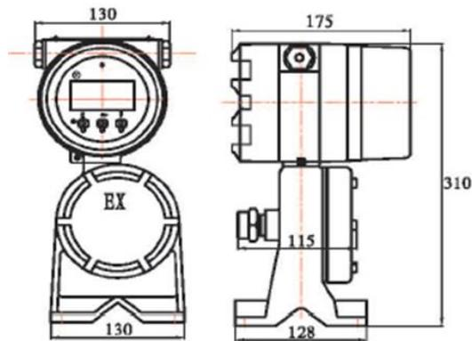
Drawing 6: Dimensions for remote type transmitter (unit: mm)
