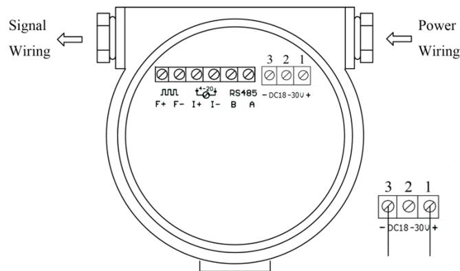
Drawing 14: DC Power Wiring
