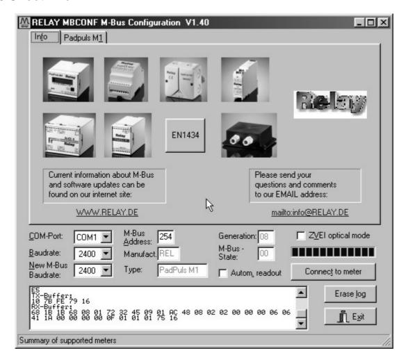
This sheet shows some photos of supported M-Bus devices from the product range of the Relay GmbH, the PadMess GmbH and further manufacturer. Here are also links to the Internet page, from which the current version of the program can be downloaded, and to the email address for criticism and suggestions to the program.
