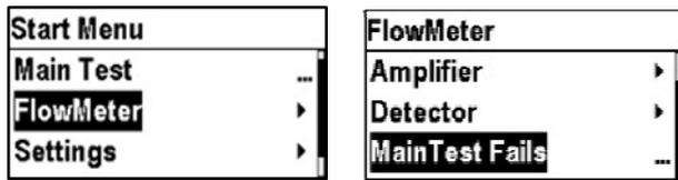
Shows the test result of the last main test.
