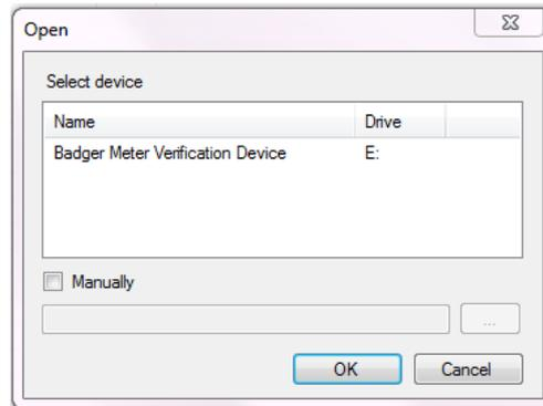
4. The measurements are automatically downloaded to the PC. You will be asked if the measurements which are on the Verification Device should be deleted or not.
