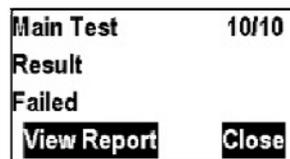
11. If the test failed, press the function key on the upper left "View Report" to see the results. See example below.
