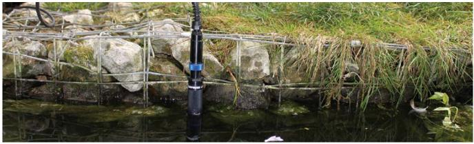
The AP-LITE is commonly used with our sapphire lensed turbidity sensor, chlorophyll sensor or blue-green algae sensors. Whilst the package includes an Aquameter the AP-LITE can also be used with one of our AquaLoggers for unmanned turbidity, chlorophyll or blue-green algae monitoring.
