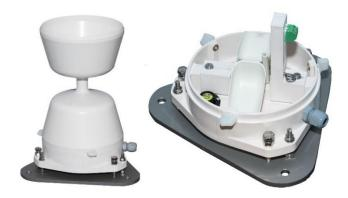
Traditional cylinder-shaped rain gauges are inaccurate due to the effect of wind blowing over the orifice. The physical presence of the gauge causes air to accelerate, carrying rainfall away from the collecting vessel. The effect of this can be up to a 20% reduction in rainfall catch. The unique aerodynamic shape of our range of scientific standard rain gauges reduces this effect, ensuring a high level of confidence in the accuracy of our measurements.
