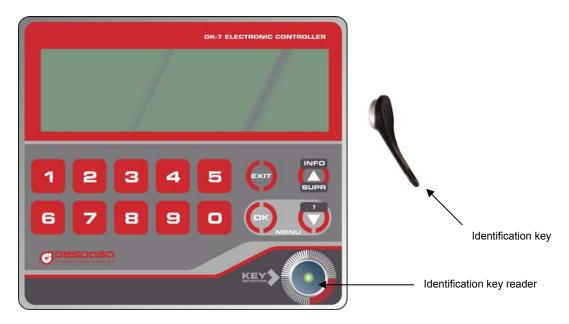
In general the numeric keys will be used for the access and data code typing, both in user and supervisor mode.
