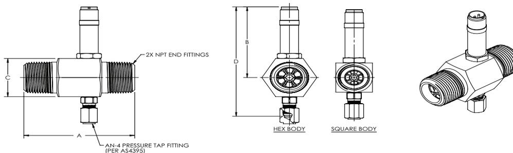
Figure 15: NPT end fitting
