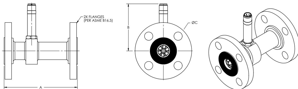
Figure 9: Flange end fitting
