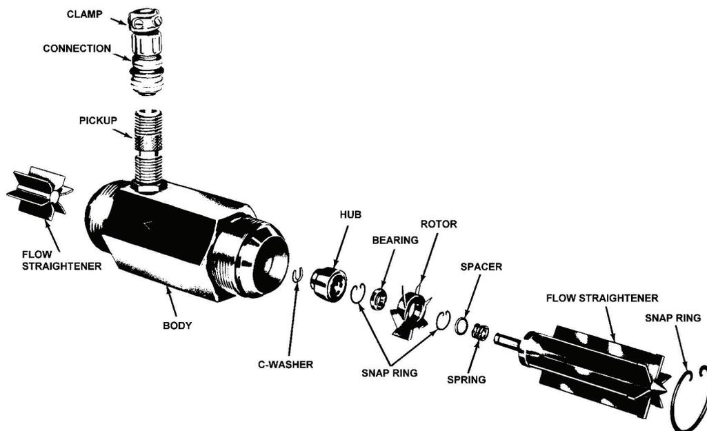
*Figure 1: Turbine flow meter*
