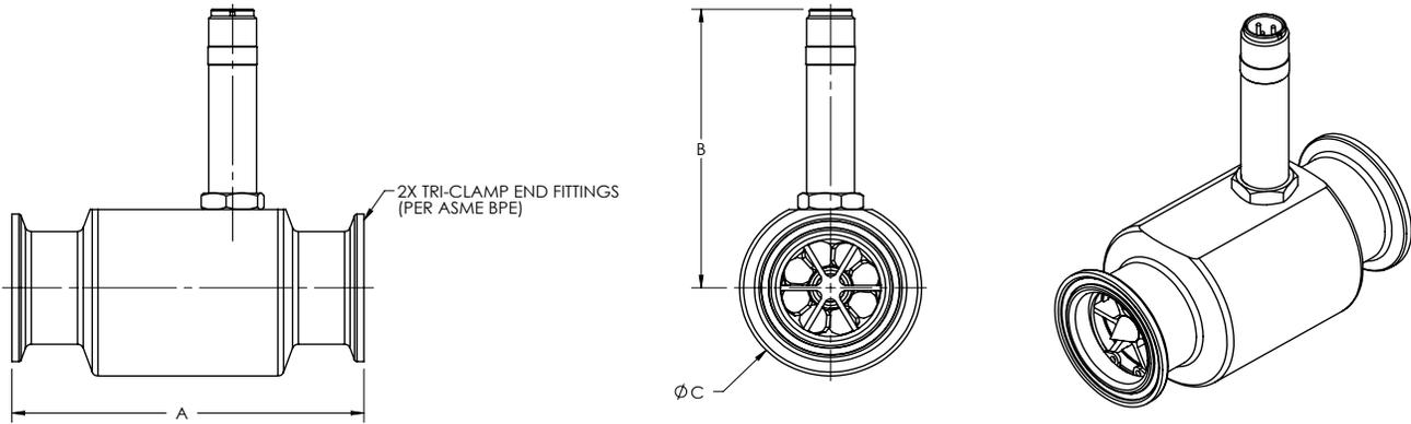
Figure 11: Tri-clamp end fitting
