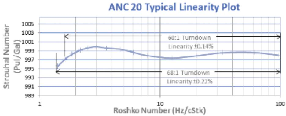
Figure 17: Typical linearity curve for a size 20 flow meter
