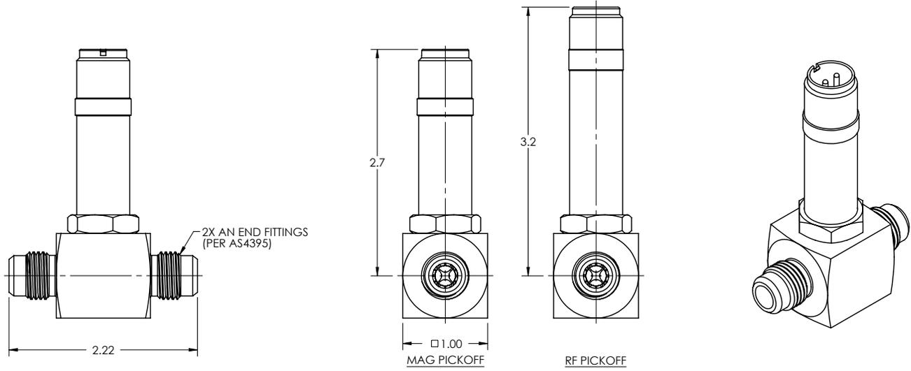
Figure 13: LoFlo meter dimensions
