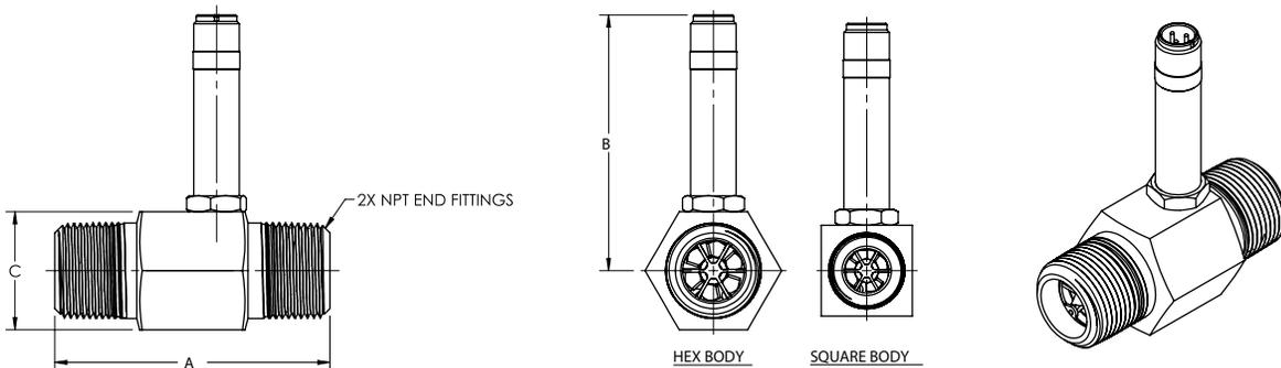
Figure 8: NPT end fitting
