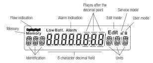
The multi-function display shows the eight-digit meter reading, along with symbols and short texts for user operation purposes.
