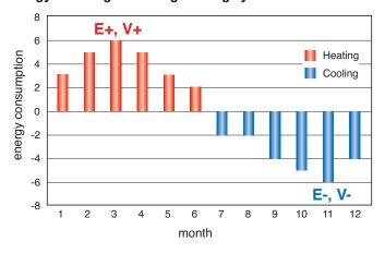
The "bi-directional energy metering" (BDE) option allows emitted energy to be metered even in twin-conduit networks that perform a combined heating and cooling function. The measurement readings for heating and cooling are recorded separately for their corresponding cost-calculation purposes.
