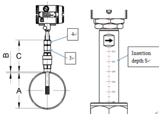
6) Use the hot tapping insertion tool to hold the flow meter
