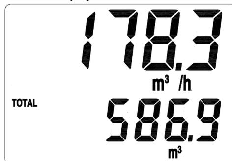
Picture 4.2 Flow rate and total flow display
