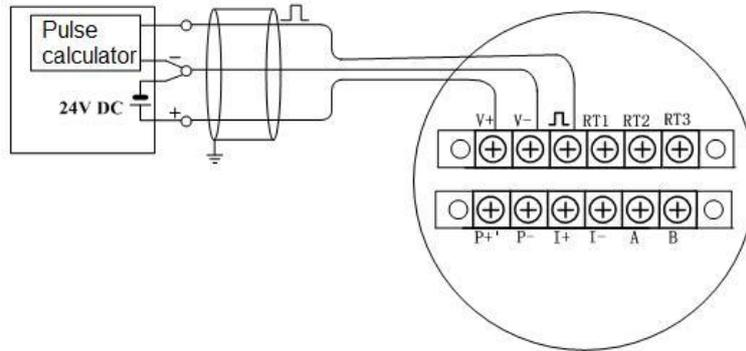
Picture 3.10 pulse output wiring on 12 terminals board
