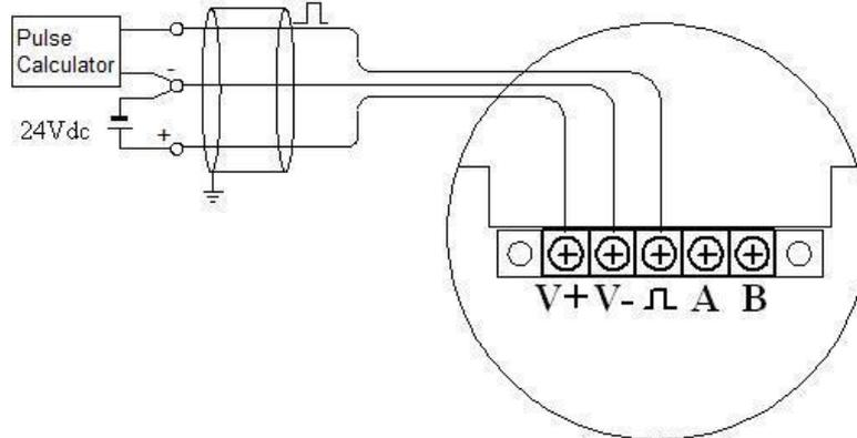
Picture 3.5 3-wire pulse output wiring on 5 terminals board
