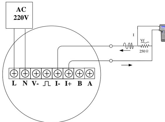
Picture 3.8 4~20mA@HART wiring on AC terminals board
