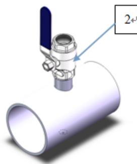
3) Drill a hole with the hot tap hole opener,  $\varnothing 22\text{mm}$  ( $\pm 0.5\text{ mm}$ ). (Please reference to the manual of hot tap mounting for details)
