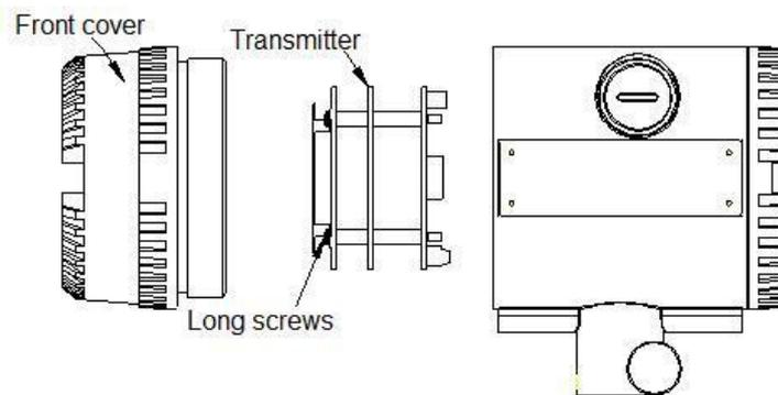
Picture 8.2 Replace the transmitter
