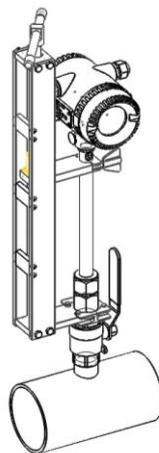
7) Adjust the direction of the flowmeter: Make sure the direction mark on the probe (Part No.5) is pointing to the direction as the flow goes. Please reference to the picture below.
