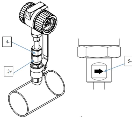
8) Open the ball valve, please make sure that procedure 1~7 is operated properly before opening the ball valve. The sleeve should be connected to the ball valve tightly that the meter can not be ejected out.
