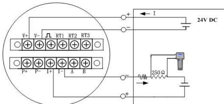
Picture 3.12 4-wire 4~20mA@HART wiring on 12 terminals board
