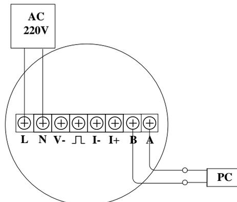
Picture 3.9 RS485 wiring on AC terminals board
