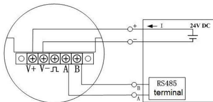
Picture 3.6 RS485 wiring on 5 terminals board
