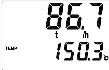
Picture 4.3 Mass flow and temperature display
