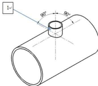
2) Connect the 1" ball valve (Part No.2) with FNPT threads on both ends to the socket. Seal the thread connection with thread sealant. Please note the lever on the ball valve should be point to up when the valve is open.
