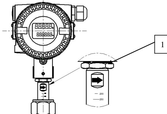
Picture 8.1 Change the transmitter's direction
