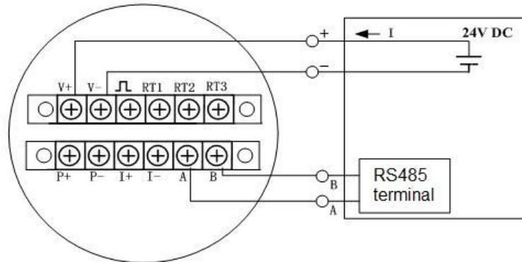
Picture 3.13 RS485 wiring on 12 terminals board
