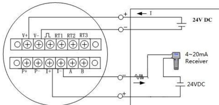
Picture 3.11 4-wire 4~20mA wiring on 12 terminals board
