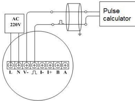
Picture 3.7 Pulse output wiring on AC terminals board
