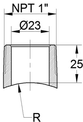
Remark: R is the outer shape of the pipeline. The material can be same as the piping if required so. If customer's chosen model require 1" NPT, than will need 1" socket base
