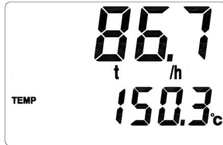
Picture 4.4 lower row is displaying temperature
