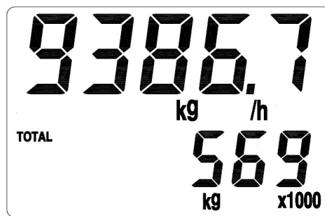
Picture 4.6 Displaying the left digits, a “x1000” mark is displayed
