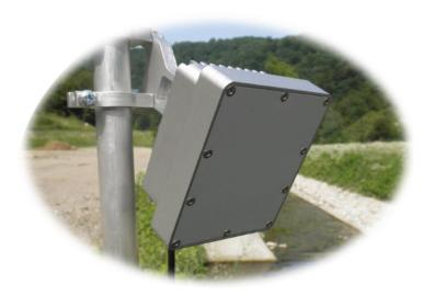
RVS-30 is a non-contact 24.125/24.200 GHz RADAR based velocity sensor that uses Doppler Effect to produce velocity data of a moving surface. The measurement can be widely used for hydrological monitoring, flood control, and environmental pollution monitoring.
