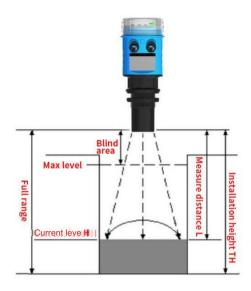
(Installation principle schematic)
