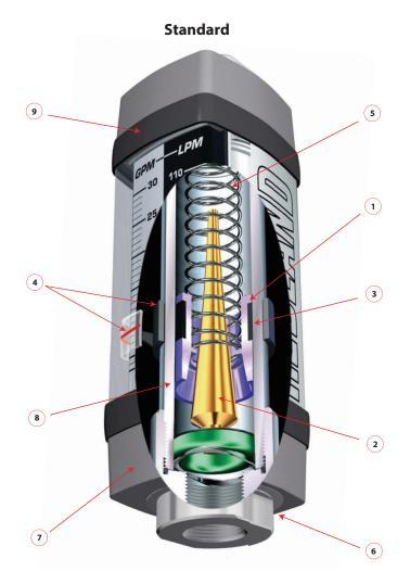
The flow meter is a variable area instrument. A sharp-edged orifice, located within the piston assembly, forms an annular opening with the contoured metering cone. The piston assembly carries a cylindrical PPS/ceramic magnet that is magnetically coupled to an external indicating magnet which moves precisely in direct response to movement of the piston. A calibrated spring opposes flow in the forward direction.
